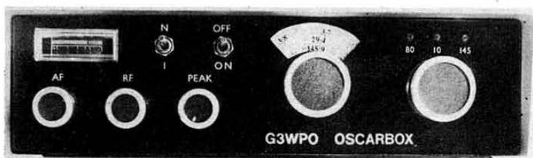
Front panel of the Oscarbox showing S-meter, af and rf gain controls, normal and inverted sideband selector switch, peak (clarify) control, main tuning dial and bandspread, and led-indicated band selector switch
